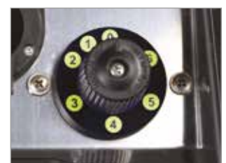
ROTARY KNOB FOR STEAM QUANTITY CONTROL
