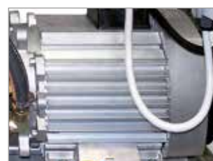
MAINTENANCE-FREE ELECTRIC MOTOR, AIR-COOLED AND PROTECTED WITH THERMAL CUTOFF
