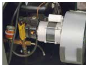
SINGLE PHASE BURNER MOTOR CONNECTED TO FAN AND DIESEL FUEL PUMP
