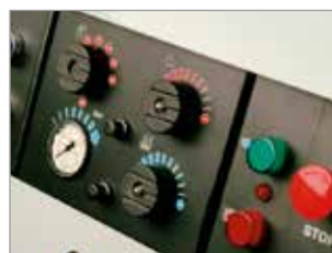
CONTROL PANEL PROVIDED WITH EMERGENCY SHUTDOWN
