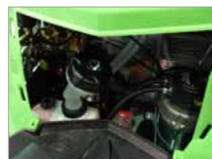
EASILY ACCESSIBLE ANTISCALE TANK
