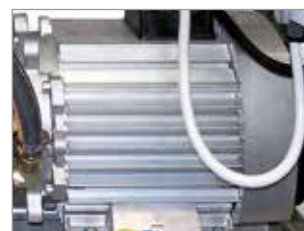
MAINTENANCE-FREE ELECTRIC MOTOR, AIR- COOLED AND PROTECTED WITH THERMAL CUTOUT
